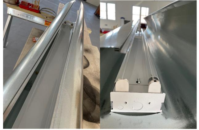
16) Take the fan assembly and insert it into the duct with the smooth end. Orient the fan such that it is blowing DOWN the tube. Take care not to install it backwards. You will want to orient the power connector of the fan to the bottom. The power connector of the fan should be in line with the power lead for the light troffer. Then use a self tapping screw, drill into the sides of the duct. Place a screw on either side. You only need two screws to hold the fan assembly to the duct.
