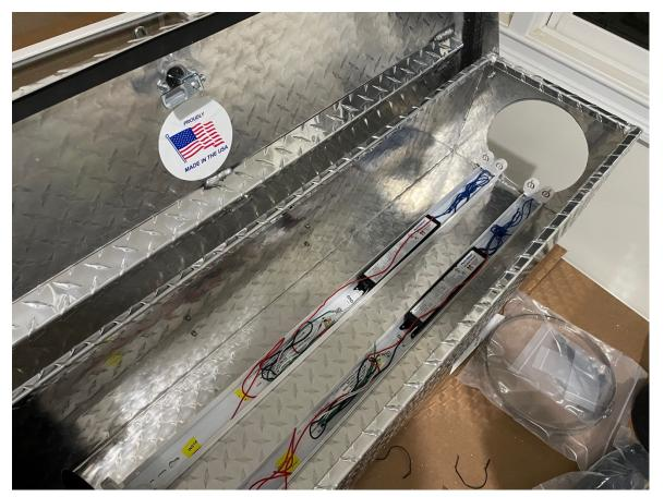
7) Note the position of the fan. Then, from the underside of the box, drill four self tapping screws through the underside of the box until it engages and eventually drills through the metal plate that the fan is connected to.
