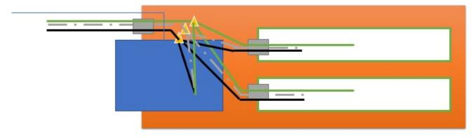
Lightbox wiring diagram. Legend: Blue box – fan; Orange box – aluminum box; Green boxes – light fixtures; Black line – supply ("hot"); Grey dashed line – white "neutral"; Green line – ground ("earth"); Yellow triangle – wire nuts; Thin blue line – fan power control cable; Gray boxes – wire connector.
